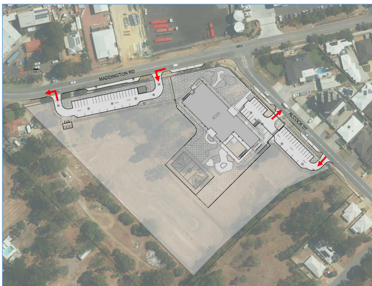
Figure 12: Vehicle Access Arrangement
